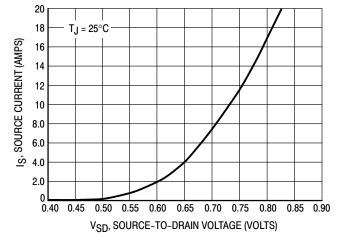
Figure 10. Diode Forward Voltage versus Current
