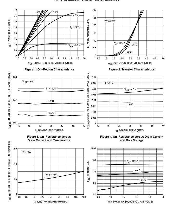
Figure 5. On–Resistance Variation with Temperature
