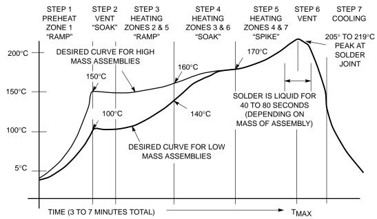
Figure 18. Typical Solder Heating Profile
