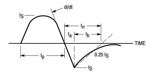
Figure 15. Diode Reverse Recovery Waveform
