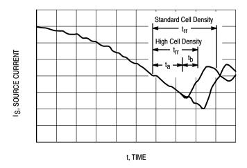
Figure 11. Reverse Recovery Time (t<sub>rr</sub>)
